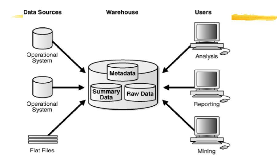
shows a simple architecture for a data warehouse. End users directly access data derived from several source systems through the data warehouse.
